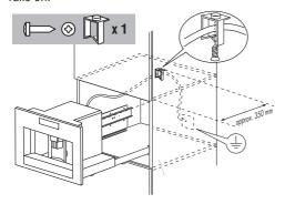
Fix the power cable with the clip.
