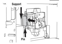
**N.B.!** If the brewing unit is difficult to insert, you must first adapt it to the right dimensions by pressing it forcefully from the bottom and top as shown in the figure.
